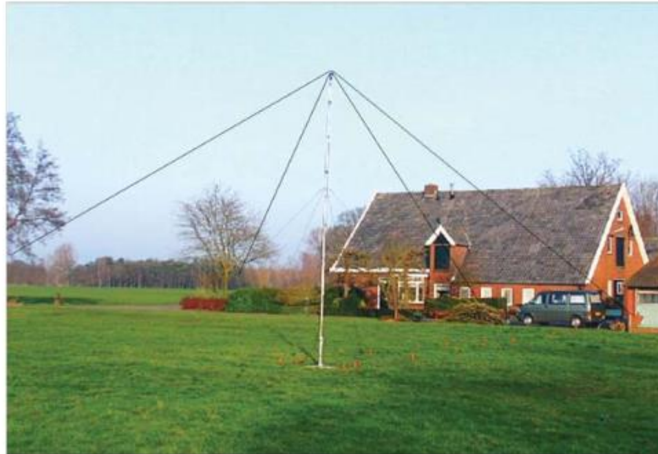
Figure 7.16 Turnstile antenna installed at the measurement location. The farmhouse and barn shown on the picture are at approximately 50 and 80 m distance. Other buildings are at >800 m distance.
